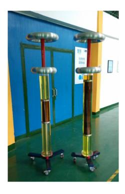
Resistive voltage dividers have very good response parameters. Therefore they are used for measurements for full and front chopped lightning impulses or impulses voltages with steep wave fronts, also in the special condition it can be used for measuring DC.
